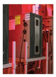
At Trane, we never settle for meeting industry standards, we strive to exceed them. So when the industry minimum testing requirement for a furnace heat exchanger is 10,000 cycles, we run it 25,000 times, subjecting it to rapid heating and cooling that will uncover any weakness in design or materials. It's harsh, but it's worth it. Because we build Trane furnaces to last, not just in the lab, but in your home.
